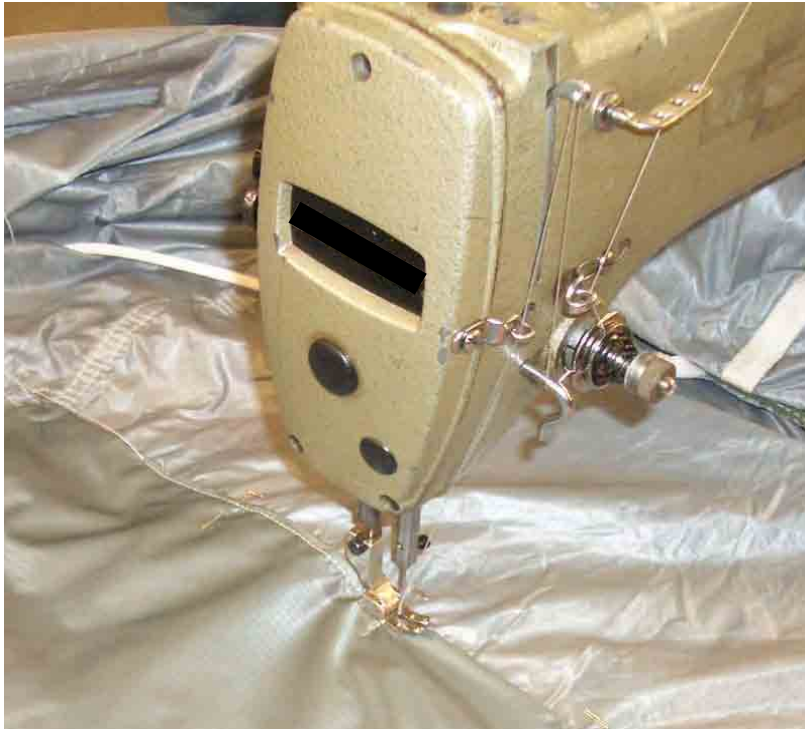
Figure 5. Sewing New Material to Damaged Panel.
