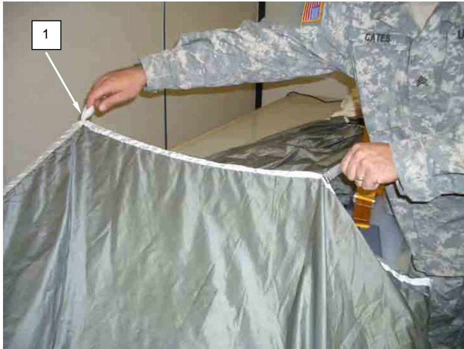
Figure 21. Folding the Top of the Canopy.
