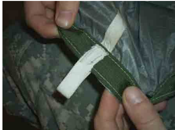
Figure 3. Attach New Suspension Line Loop (Bartack Option Shown).
