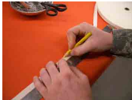
Figure 1. Measure the Damaged Area.
