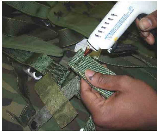
Figure 10. Apply Glue to the Upper Main Lift Web.
