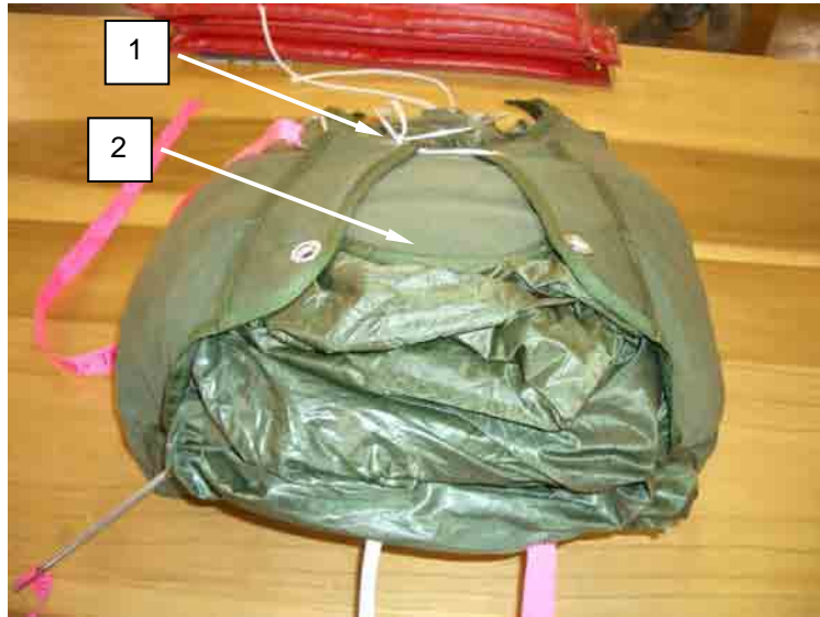
Figure 53. Inserting Temporary Pin and Placing Protection Cap.
