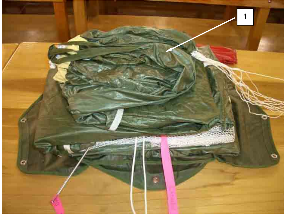
Figure 49. S-Folding Remaining Canopy.
