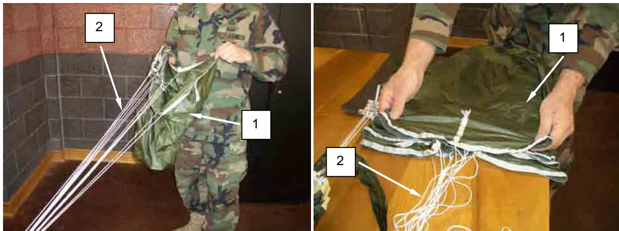
Figure 29. Folding the Extractor.
