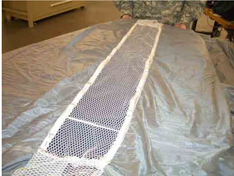
Figure 4. Centering New Mesh Panel over Opening and Securing with T-pins.
