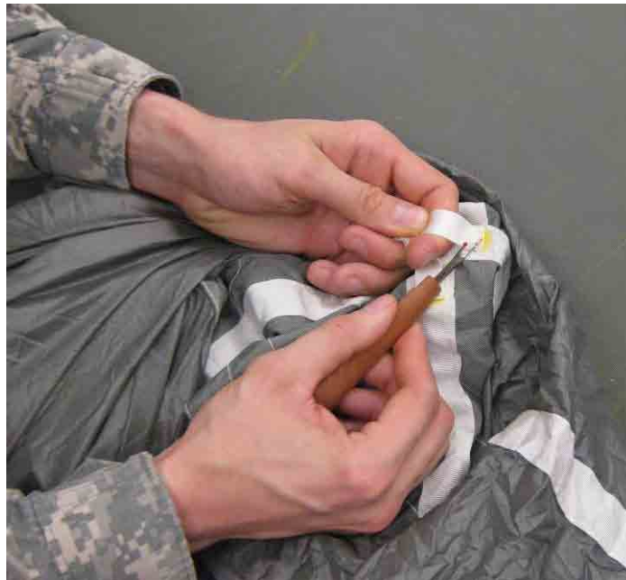
Figure 1. Removing the Damaged Apex Bridle Attachment Assembly.
