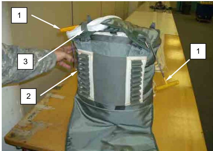
Figure 46. Make First Locking Stow.
