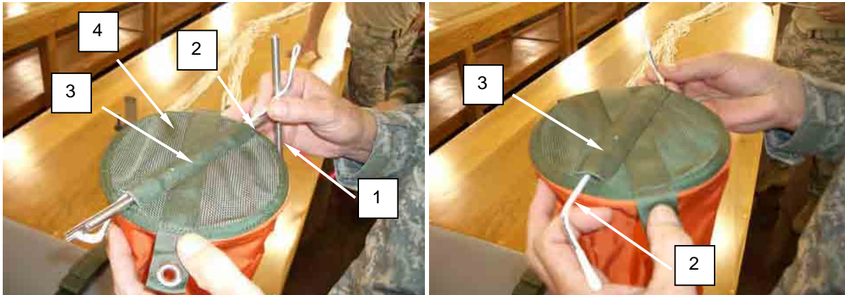
Figure 2. Assembling the Ejector Spring.
