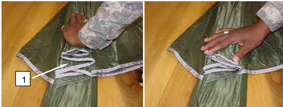
Figure 25. S-Folding of the Top Right Side of the Apex Scoop.
