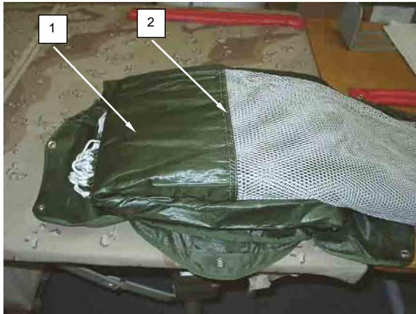
Figure 44. Making First S-Fold.
