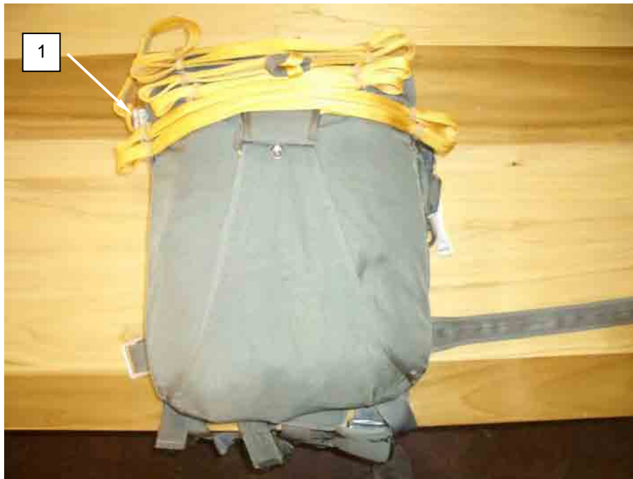
Figure 62. Continue Stowing Static Line across the Top of the Pack Tray (shown with Static Line Extension).
