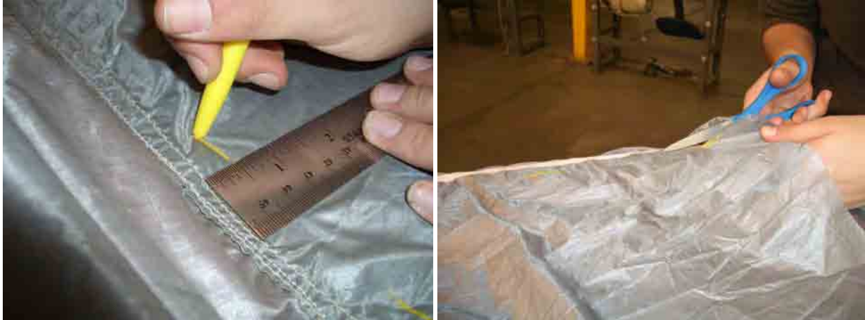
Figure 7. Removing Damaged Panel.
