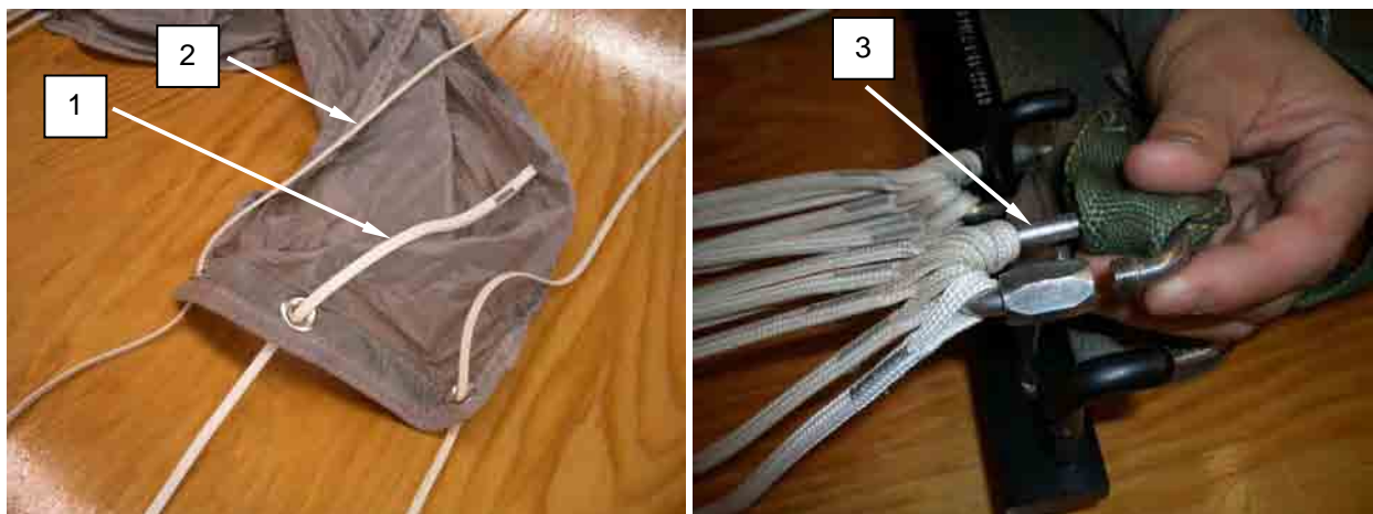
Figure 1. Replacing a Main Canopy Suspension Line.
