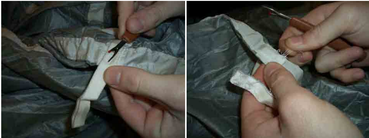
Figure 2. Removing Damaged Packing Loop with Stitch Removal Tool.
