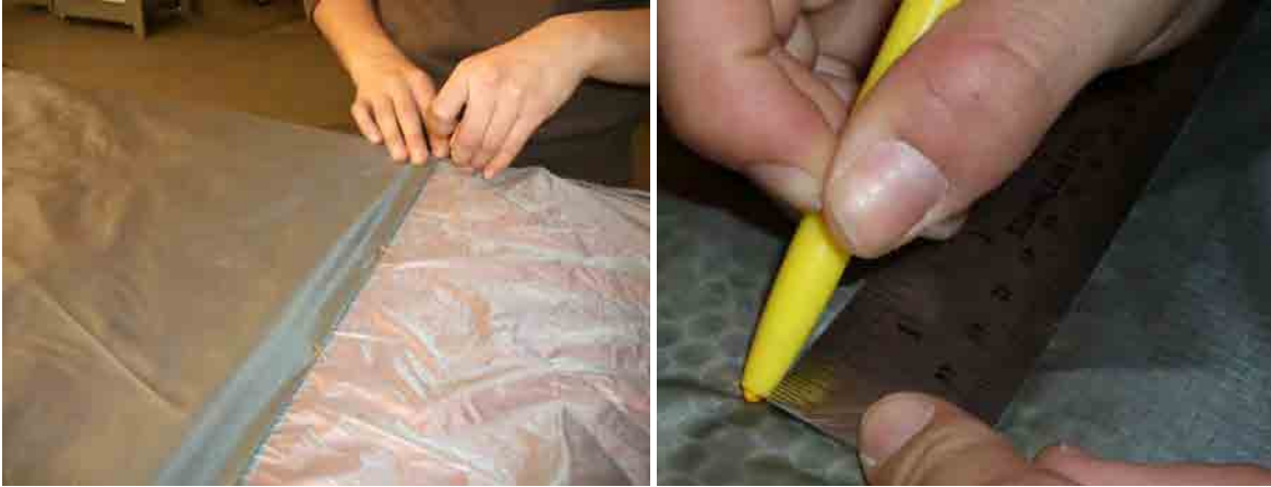
Figure 3. Centering and Pinning New Material to Damaged Panel.
