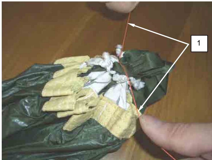
Figure 42. Tying off Apex Loops.
