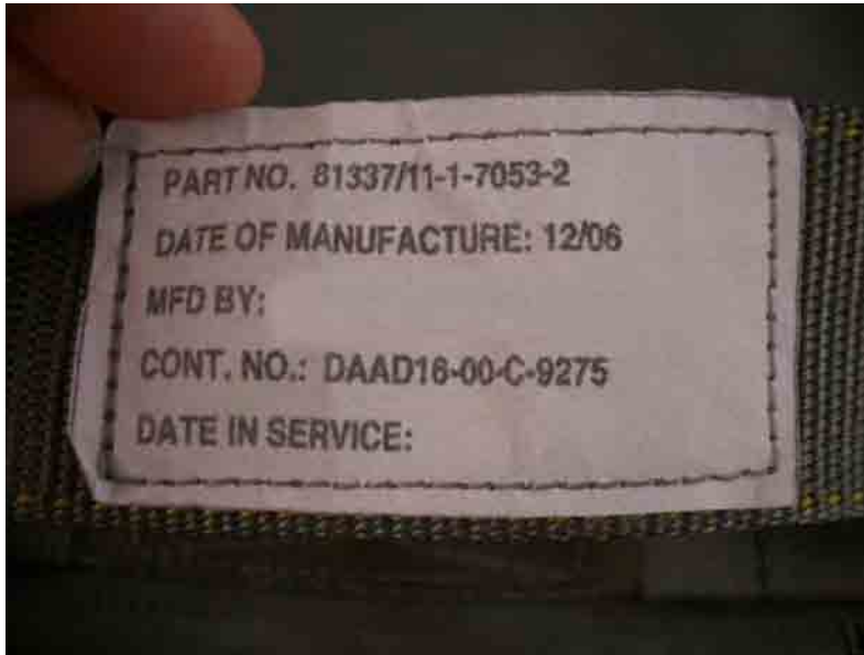
Figure 7. Enter the Date in Service on Horizontal Back Strap in Data Label.
