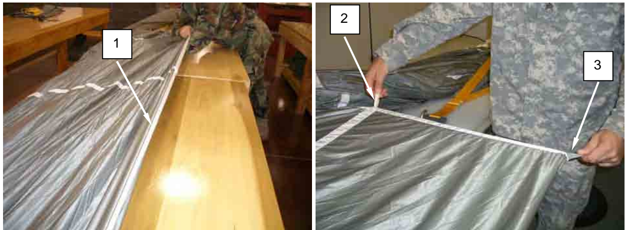
Figure 20. Pull Packing Tab from Left Side of Table to Right Side over Seam 14.
