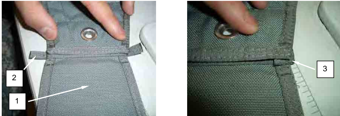
Figure 5. Replace Damaged Pin Protector Flap.
