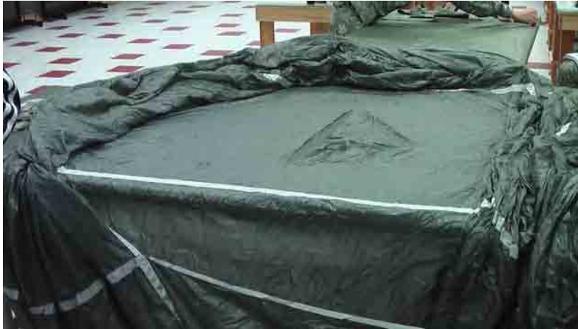
Figure 1. Inverting Damaged Panel and Securing with T-pins.
