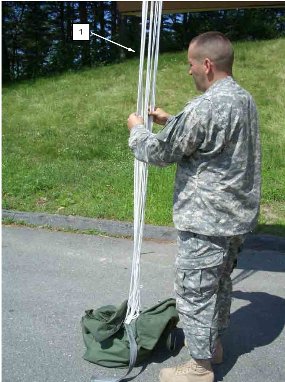
Figure 3. Clearing Suspension Lines of Debris and Removing Entanglements.
