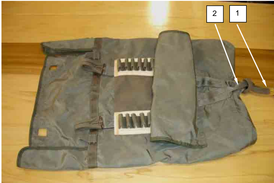
Figure 29. Securing Static Line to Deployment Bag.
