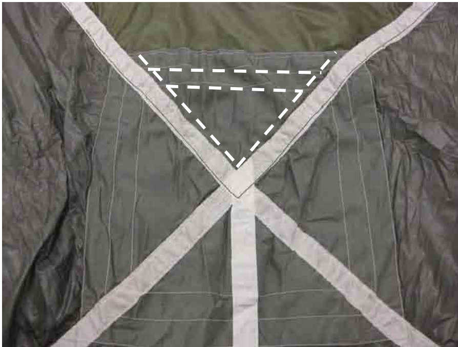
Figure 10. Stitch Over Existing Stitch Patterns.
