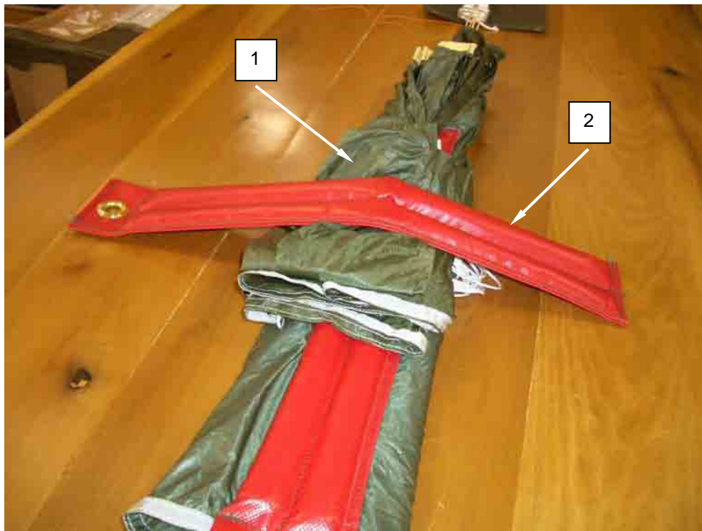
Figure 32. Placing Extractor on Top of Apex Area.
