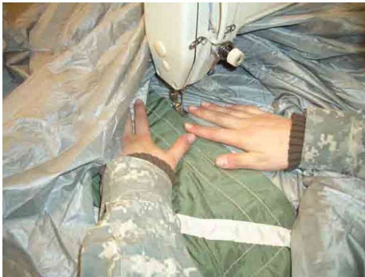
Figure 1. Re-stitching Main Canopy Reinforcement Panel.
