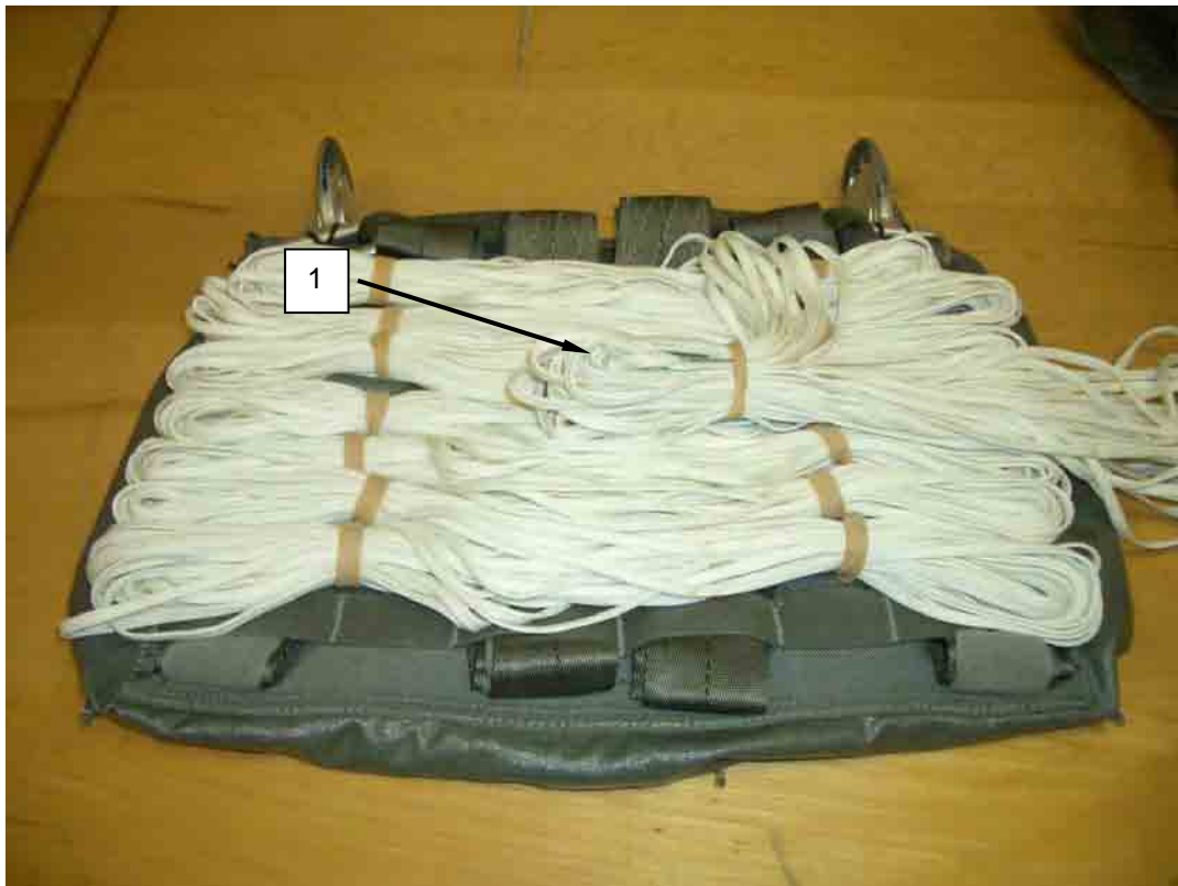
Figure 39. Placing Last Free Stow on top of Stowed Lines.
