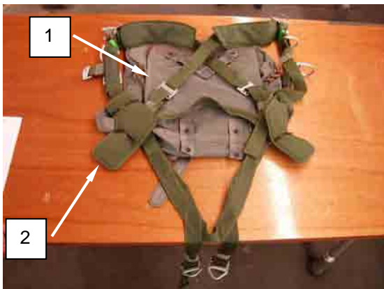
Figure 1. Remove Harness Assembly from Pack Tray.
