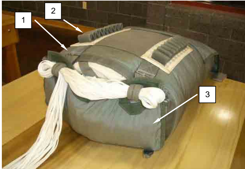
Figure 48. Flattening the Deployment Bag to Form a Wedge.
