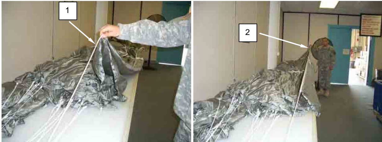
Figure 19. Flip Right Line Group over Left Line Group and Locate Packing Loop 14.
