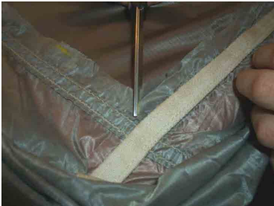
Figure 8. Cutting in Corners at 45 Degree Angle.
