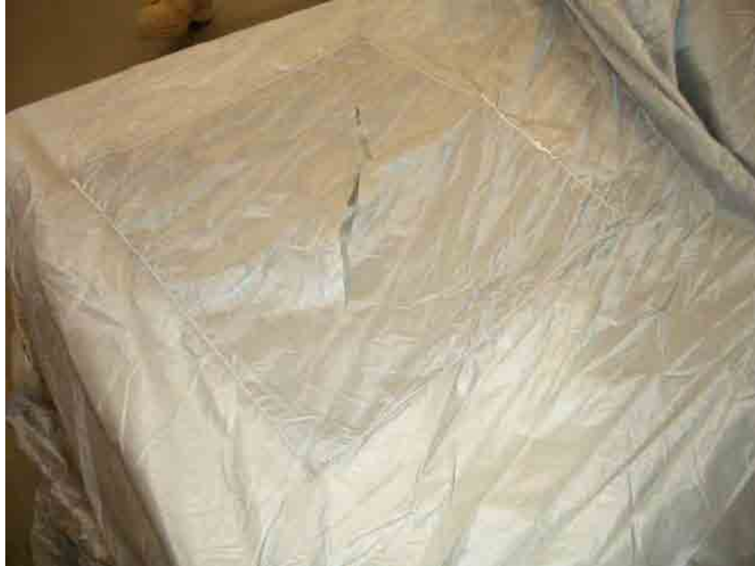
Figure 12. Re-inverting Damaged Area and Placing onto Sewing Table Patch Side Down.
