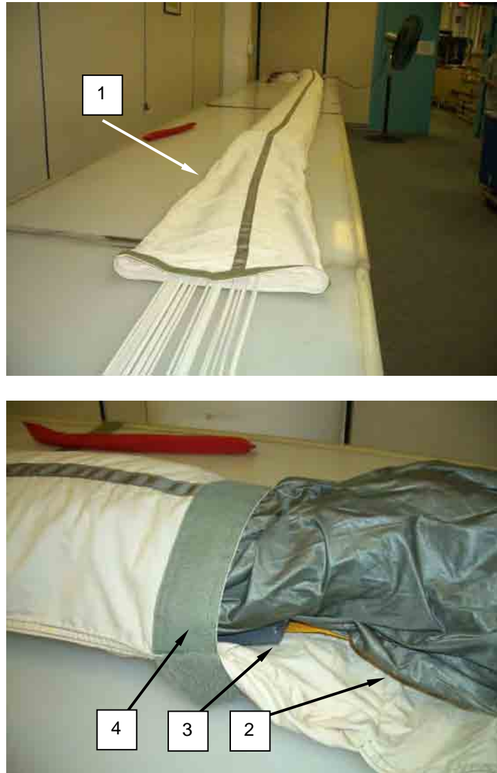
Figure 30. Pull Deployment Sleeve over Canopy.
