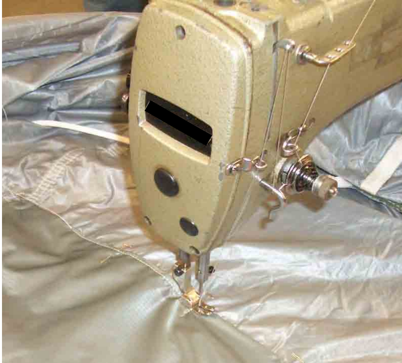
Figure 5. Sewing New Material to Damaged Panel.
