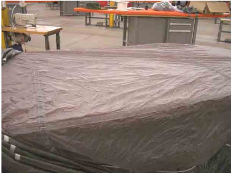
Figure 1. Inverting Damaged Panel and Securing with T-pins.
