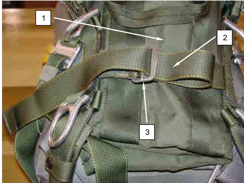
Figure 64. Connect Chest Strap to 1-inch Quick-fit Friction Adapter.
