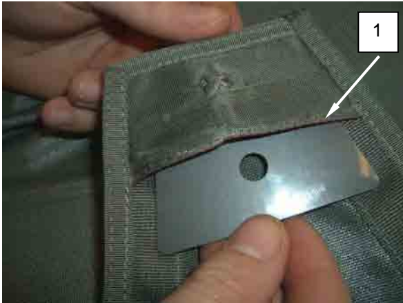
Figure 3. Insert New Stiffener.
