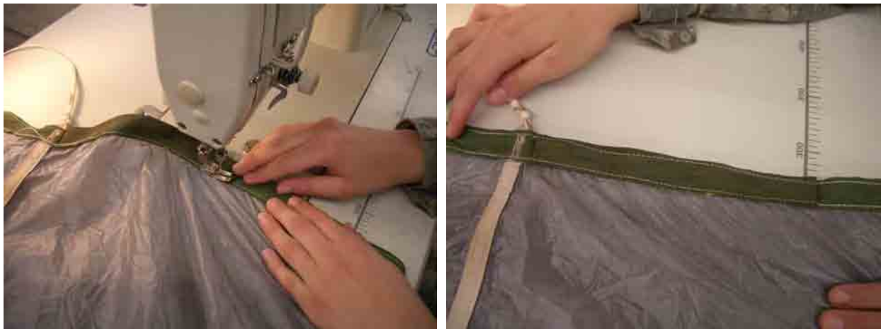
Figure 4. Sew New Material over Damaged Area.
