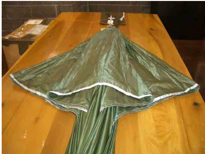
Figure 19. Folding and Dressing Left and Right Apex Scoops.
