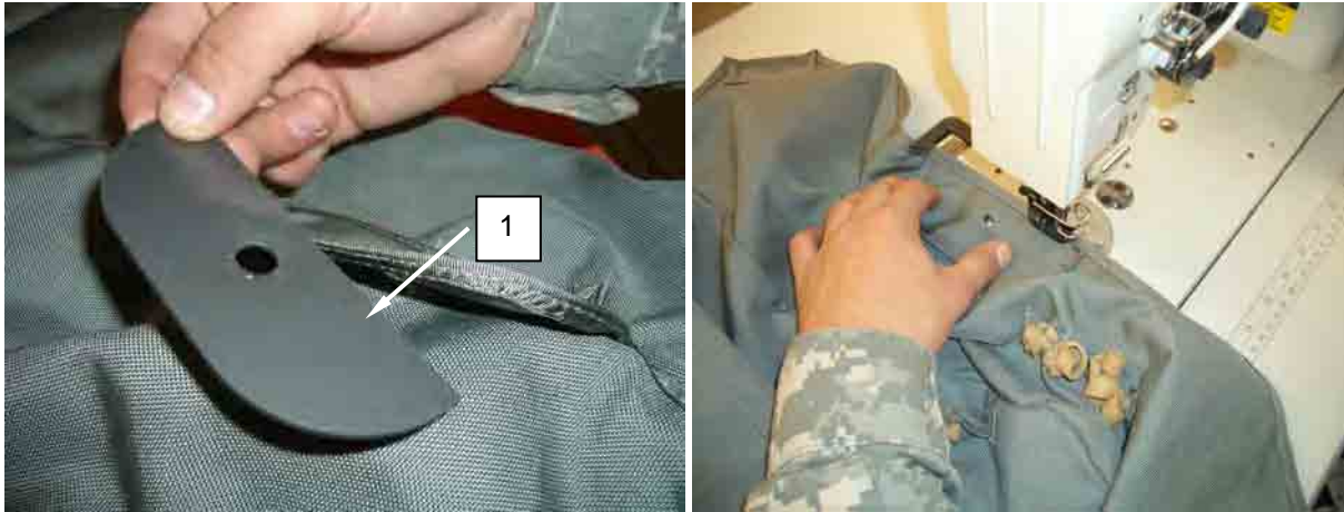
Figure 2. Insert a New Stiffener.
