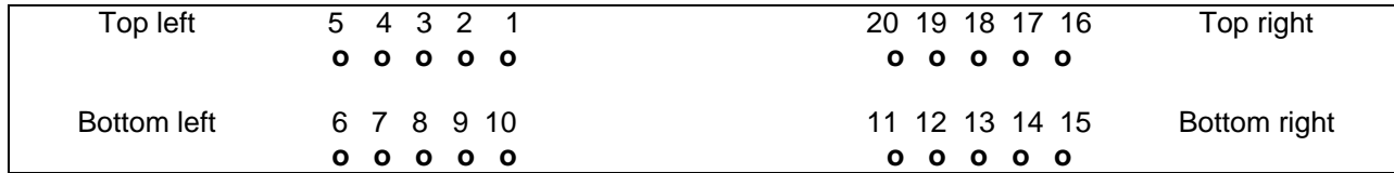
Figure 8. Suspension Line Groups.
