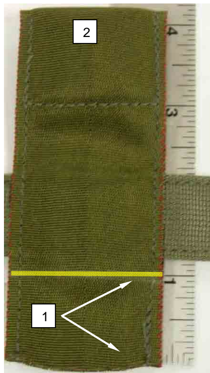
Figure 9. Tuck Tab Assembly.
