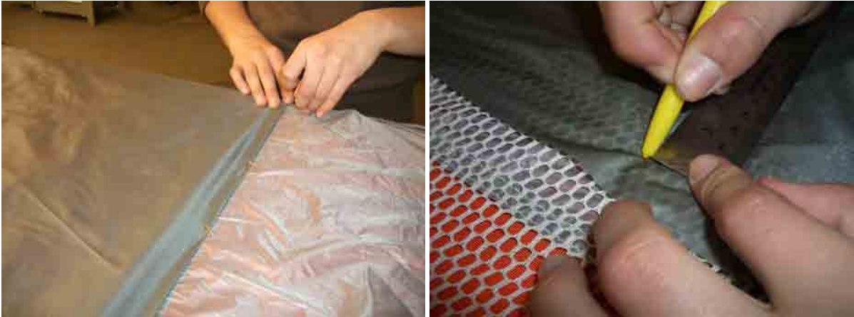
Figure 3. Centering and Pinning New Material to Damaged Panel.
