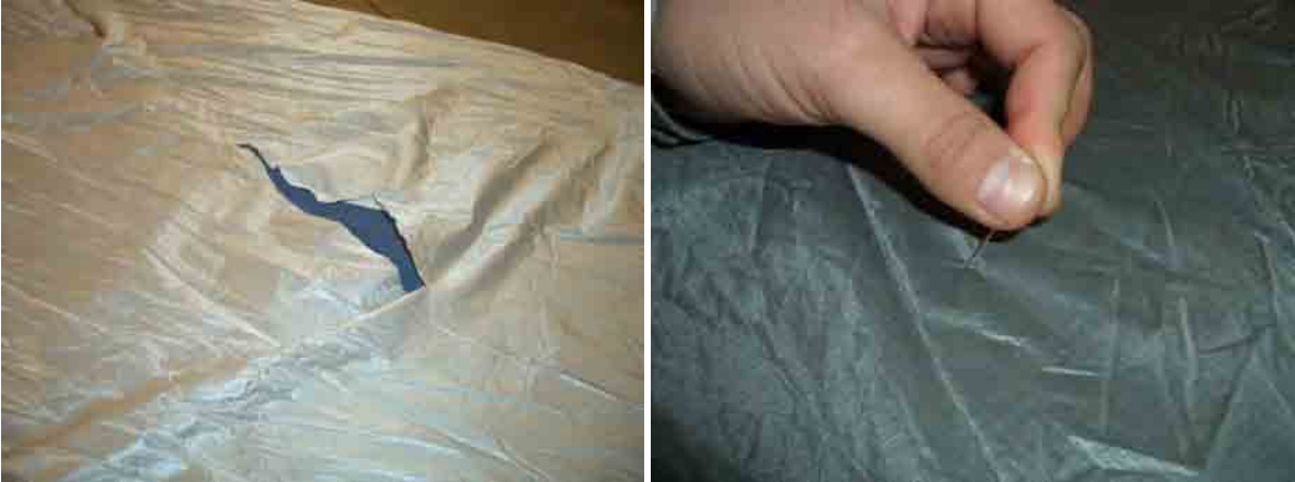
Figure 8. Inverting Damaged Panel and Securing with T-pins.
