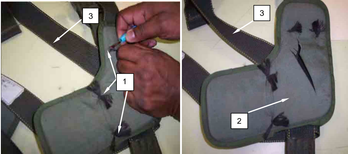
Figure 1. Removing Damaged L-Shaped Ejector Snap Pad.
