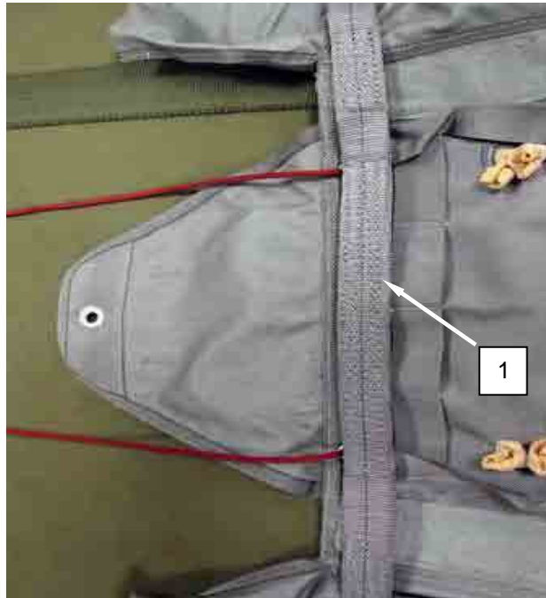
Figure 11. Centering the Spreader Bar between the Upper and Lower Grommets.
