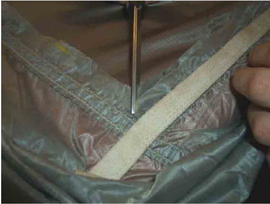
Figure 7. Cutting in Corners at 45 Degree Angle.
