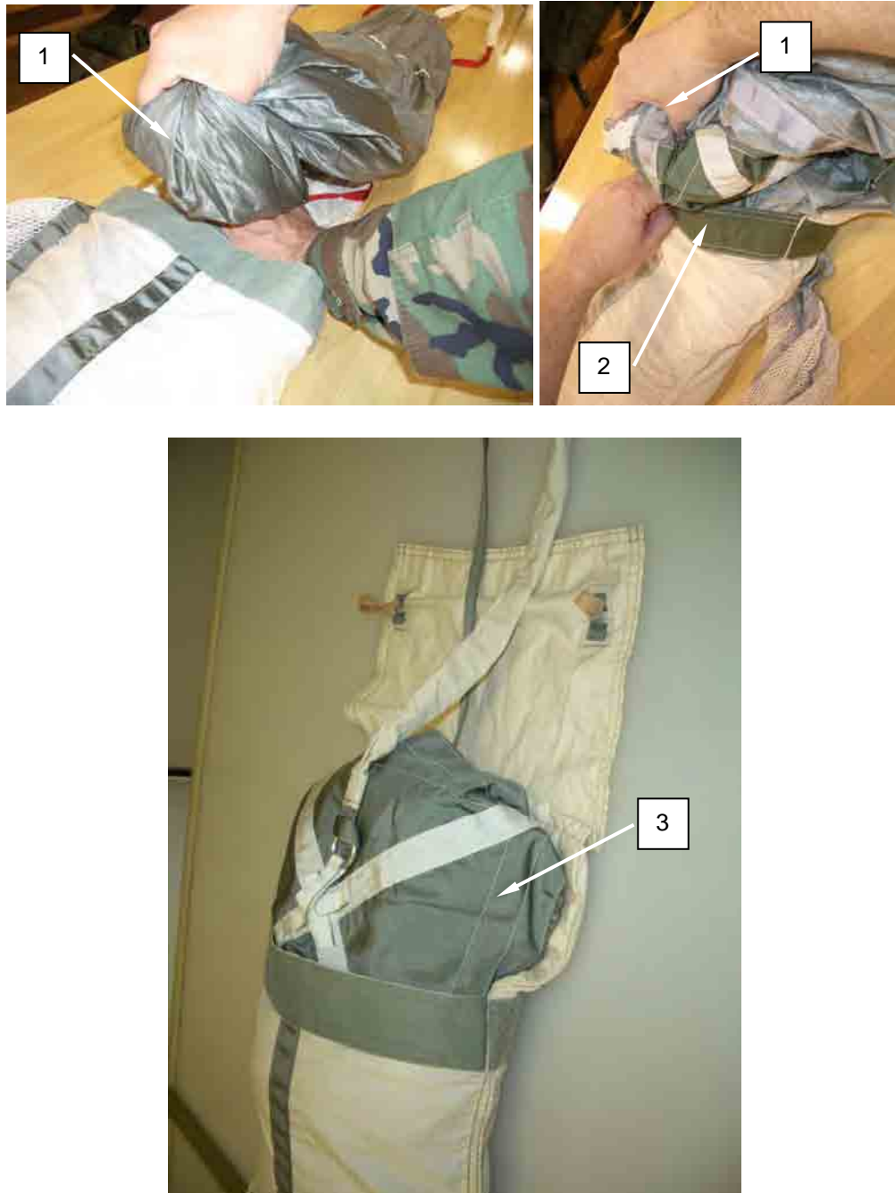
Figure 33. S-Fold Center Section Fabric.
