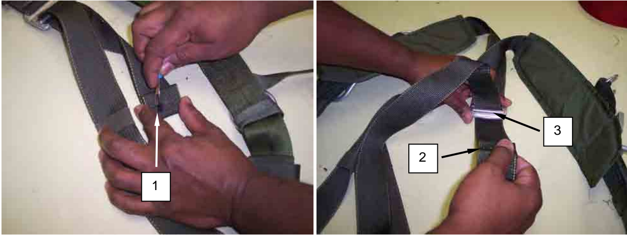
Figure 2. Remove Stitching From Diagonal Back Straps.
