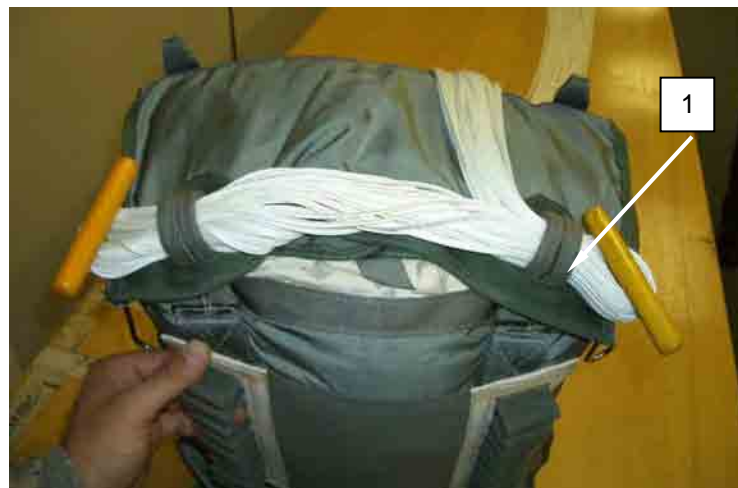
Figure 47. Make Second Locking Stow.
