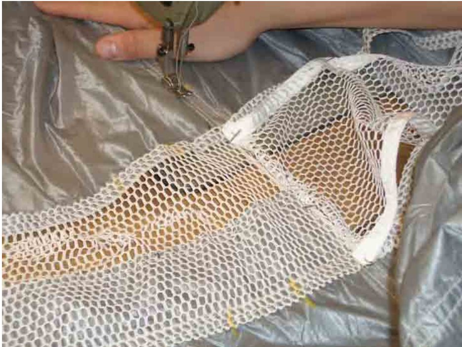
Figure 5. Sewing New Mesh Panel in Place.
