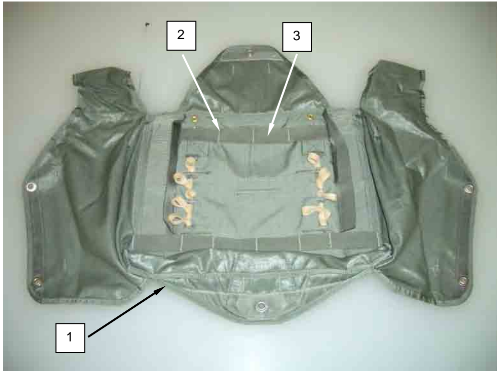
Figure 1. Remove Damaged Elastic Riser Stow Bar.
