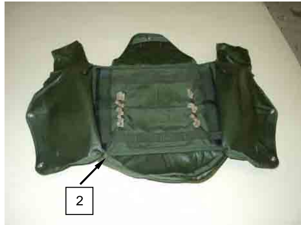
Figure 1. Remove Reserve Pack Tray from Reserve Canopy Risers.
