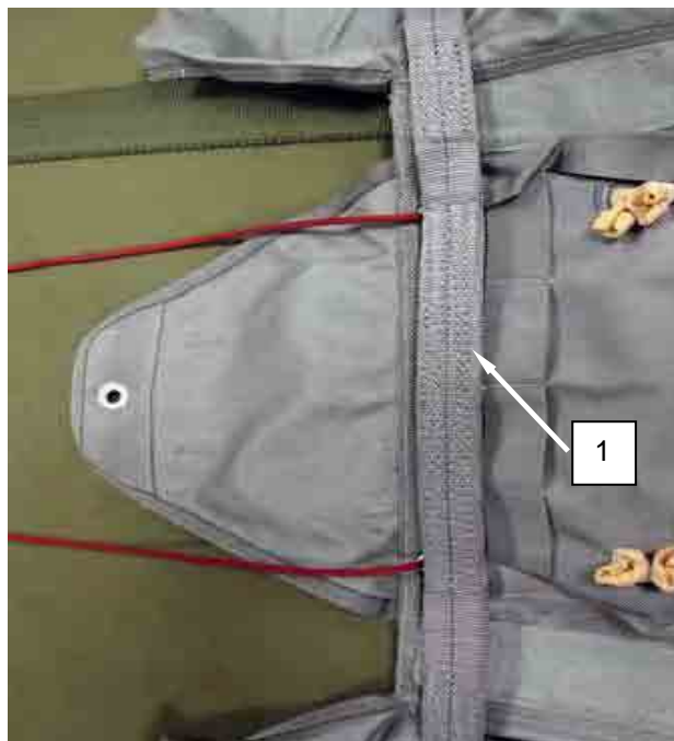
Figure 9. Centering the Spreader Bar between the Upper and Lower Grommets.
