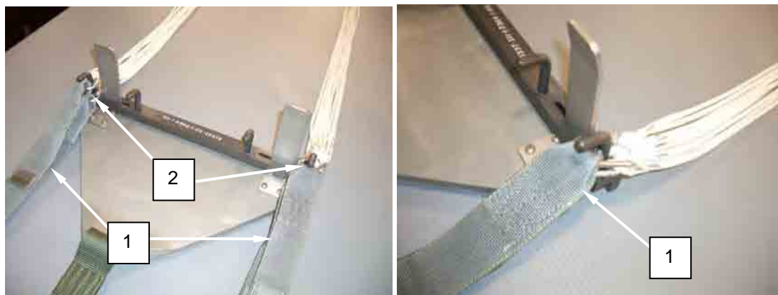
Figure 3. Attaching Risers to Connector Links.
