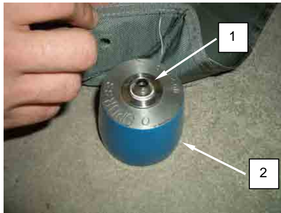
Figure 5. Position Grommet on Die with Barrel Facing Up and Place Washer over Grommet Barrel.
