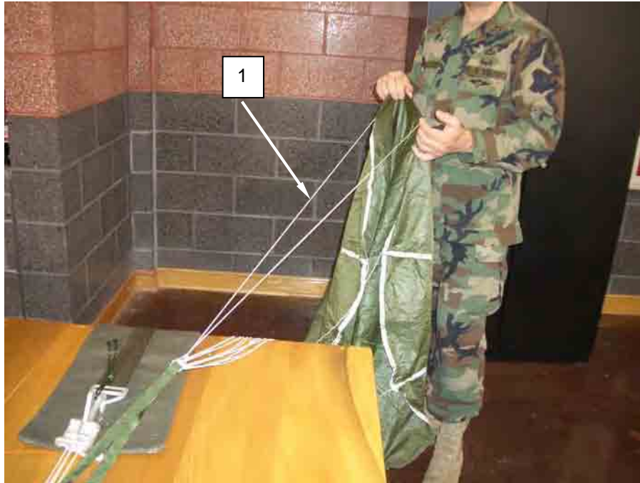
Figure 28. Perform Line Check of the Extractor.
