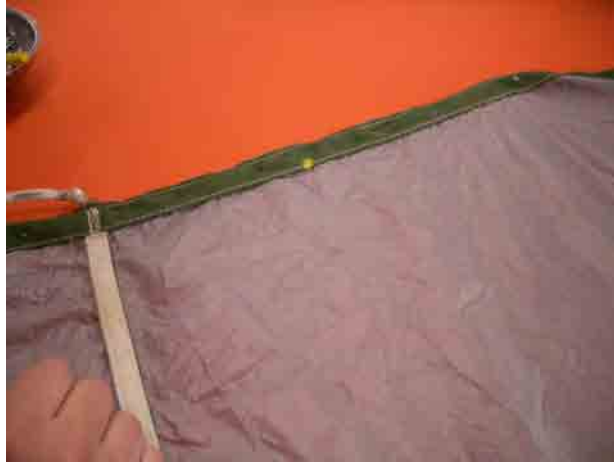
Figure 1. Smooth Out Damaged Area on a Repair Table.
