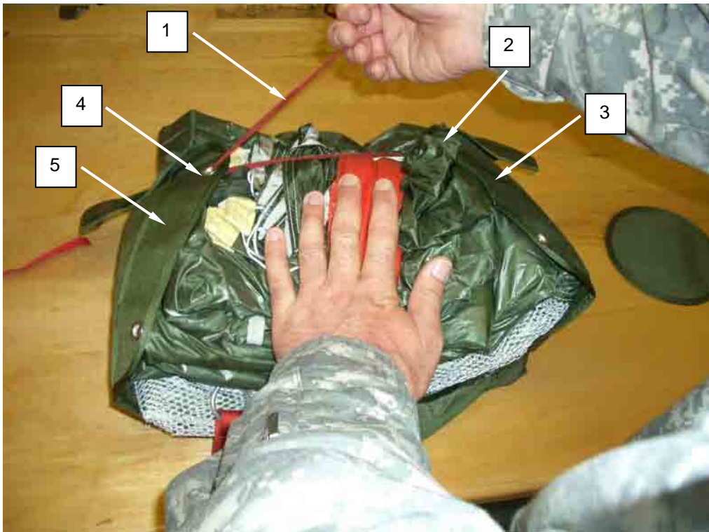
Figure 52. Placing Lower Pull-up Cord through Lower Grommet.
