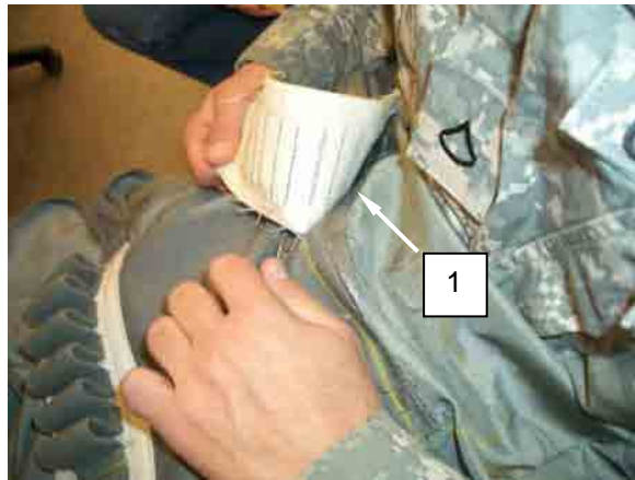
Figure 8. Remove Damaged Suspension Line Stow Loop Panel.
