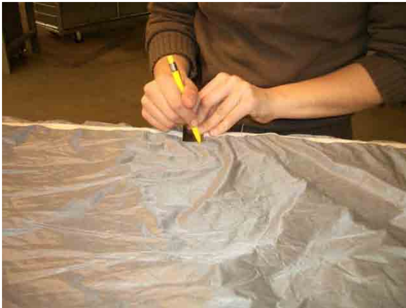
Figure 6. Re-inverting Damaged Panel and Placing on Repair Table.
