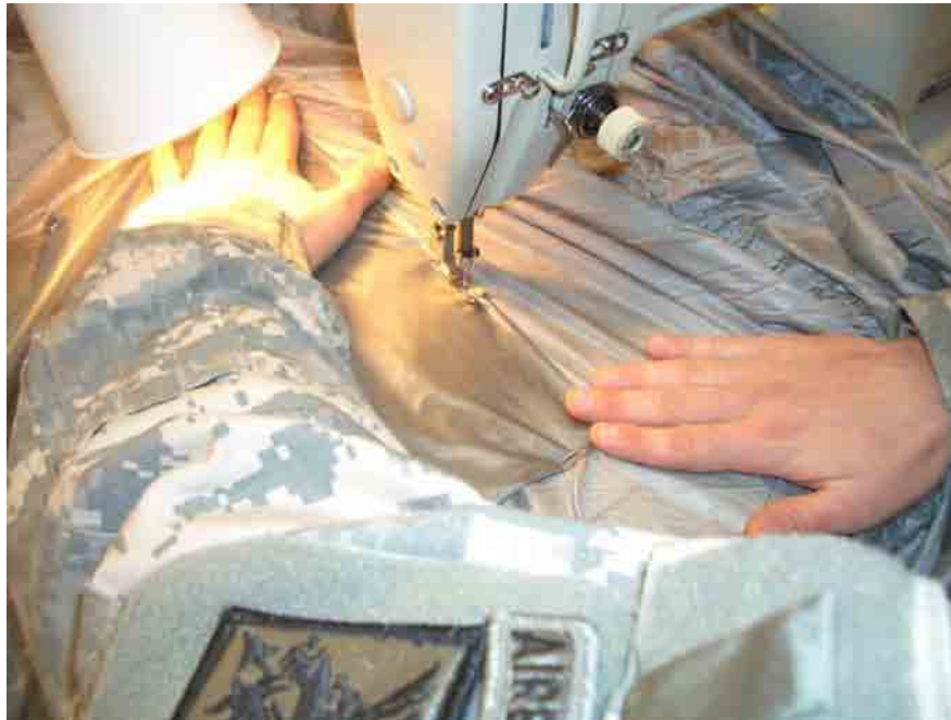
Figure 11. Sewing New Material over Damaged Area 1/16-inch from Edge.
