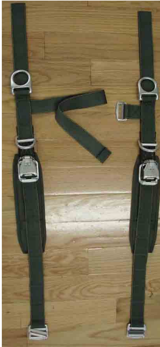
Figure 4. Right and Left Upper Main Lift Web Assemblies.
