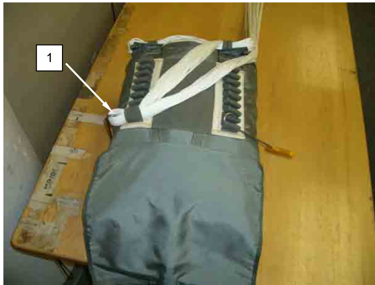
Figure 49. Make First Regular Stow.
