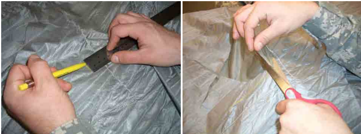
Figure 13. Marking 1-inch in from Stitches and Removing Damaged Area.
