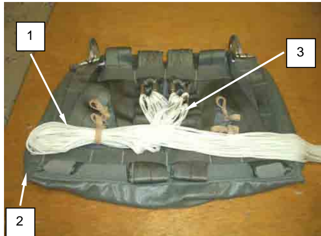
Figure 34. Making First Regular Stow.
