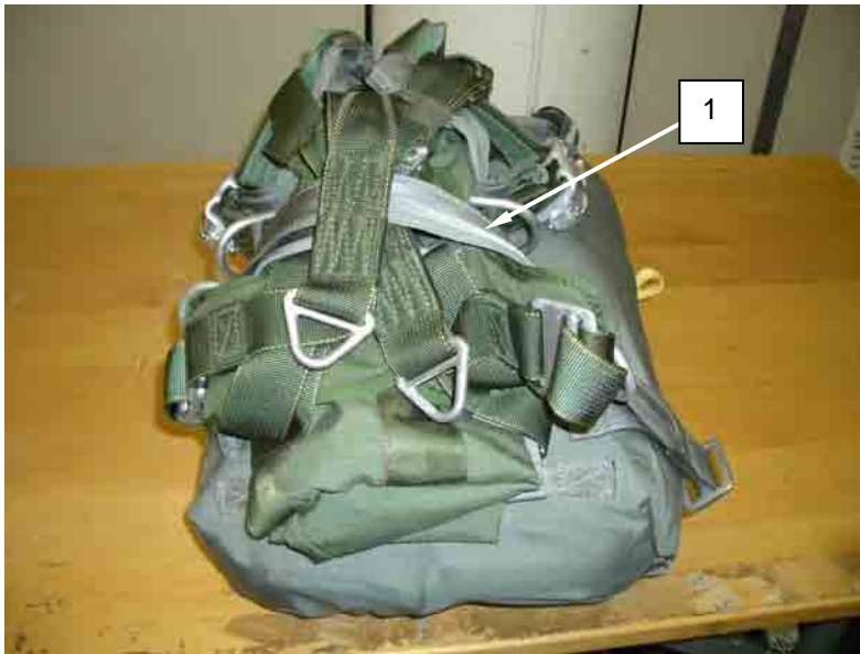
Figure 66. Route Waistband under Saddle.
