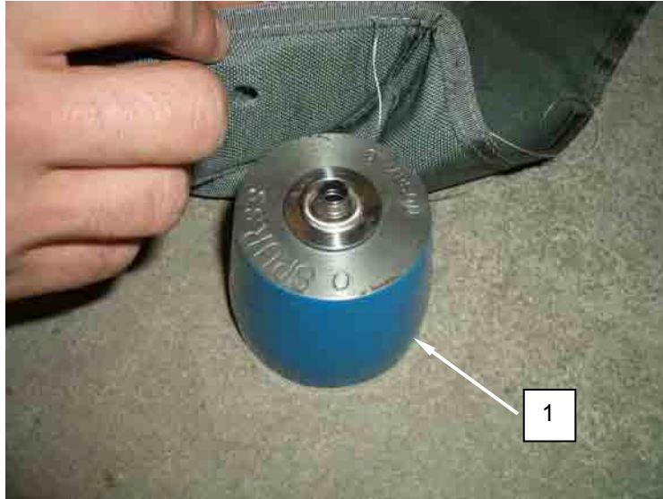
Figure 2. Position Grommet on the Die.
