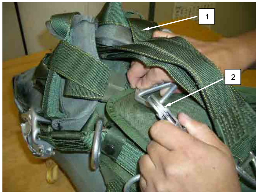
Figure 65. Attach Leg Straps to Leg Strap Quick-Ejector Snaps.
